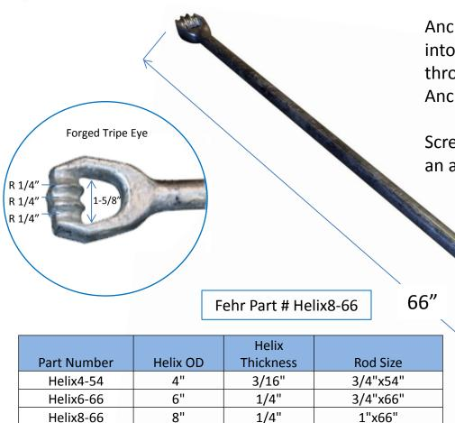
Anchors are installed by simply turning the anchor into the ground, utilizing a turning bar placed through the anchor's forged eye. No-Wrench Anchors can be installed by hand or by machine.
